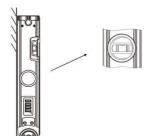
Place the bottom side of fixed blade tightly on the measured surface. If the bubble inside the vial stays between the marks on the vial's surface, the measured surface is vertical.
