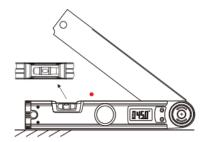
Place fixed blade on the measured surface. If the bubble inside the vial stays between the marks on the vial's surface, the measured surface is horizontal.
